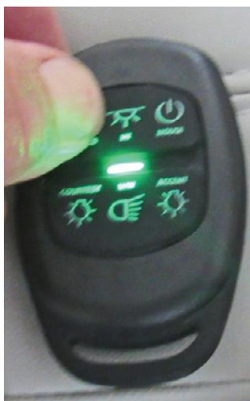
C-Zone Remote Fob, Controls Battery Switches and Lighting
