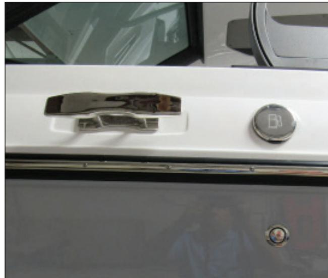
Retractable Cleat Deployed, Fuel Fill and Vent
