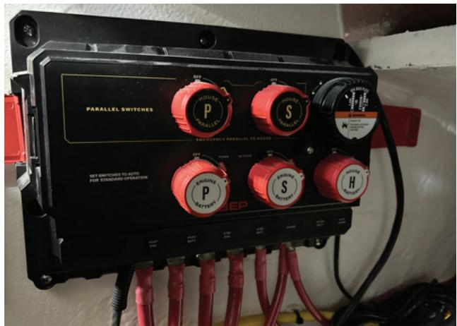
Automatic Twin Engine Battery Switches
