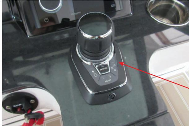
Typical Mercury DTS Joystick Control
