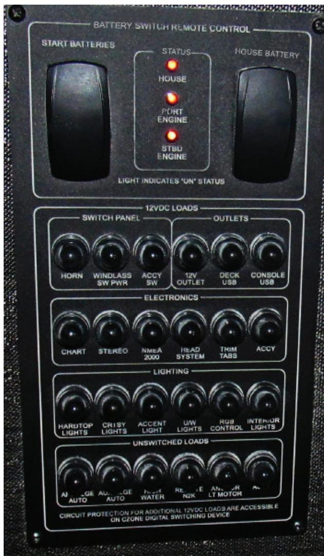
Circuit Breaker Panel And Battery Switches
