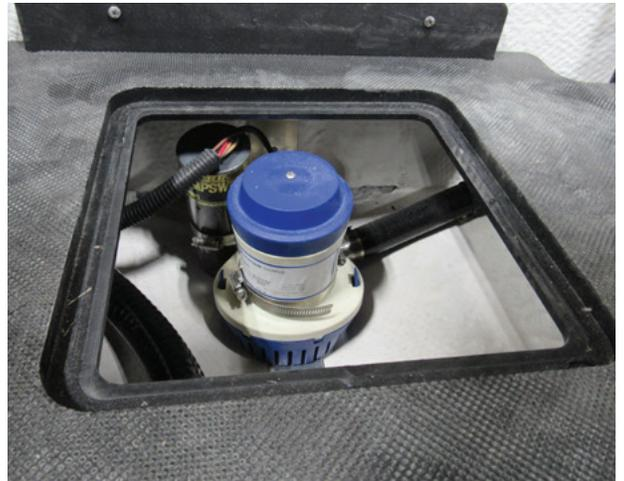
Aft Automatic Bilge Pump With Float Switch
