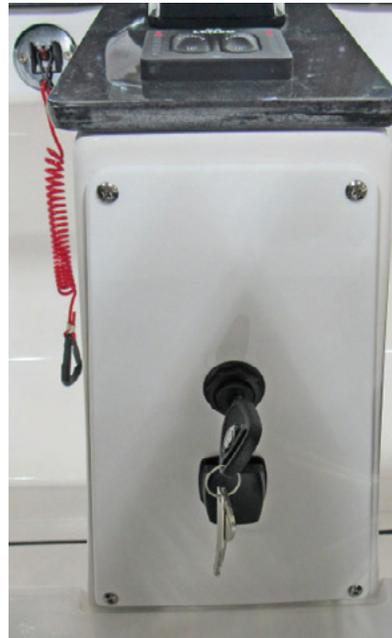
Elite 25, 27 Ignition Switch, Aft Console Face
