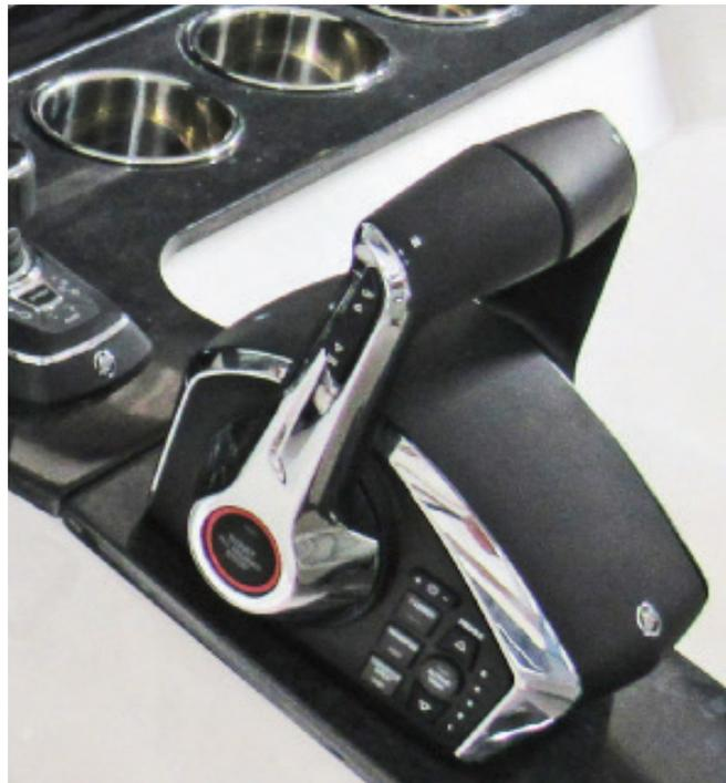
Mercruiser Twin Engine Controls With Tilt/Trim Switches
