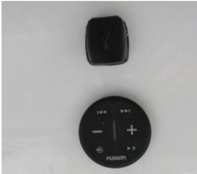
USB Charging Port and Aft Cockpit Bluetooth Stereo Remote
