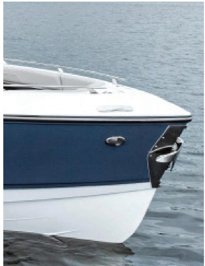
Optional Anchor Windlass and Integrated Bow Plate/Chute
