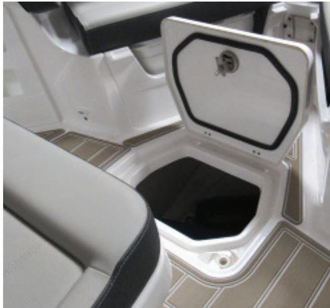
E27/E30 Bow Storage Compartment Drain/Gutter
