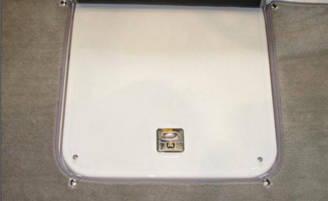
Typical Twist Lock Latch - Latched With Handle Folded Flush
