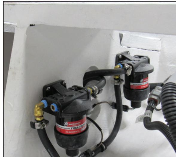
Twin Engine Fuel Filters (Elite 30)
