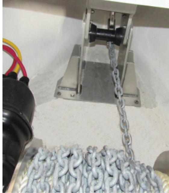
Anchor Locker With Drum Windlass
