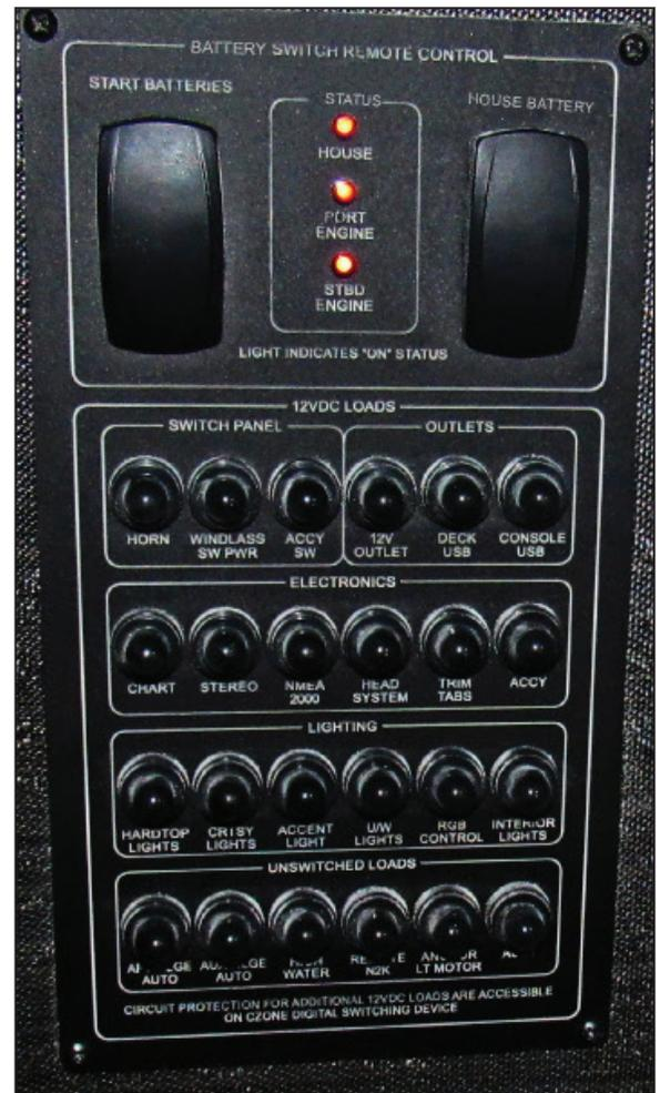
Battery Rocker Switches and DC Breaker Panel In Head
