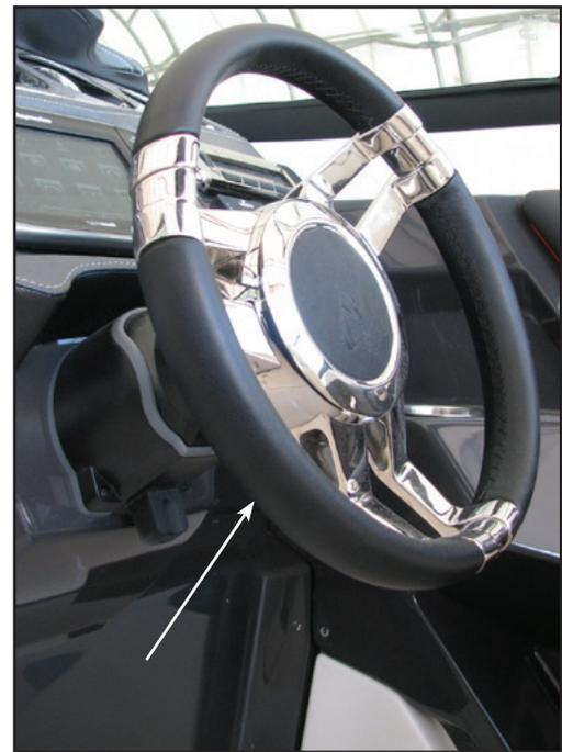
Tilt Steering Wheel & Tilt Release Lever
