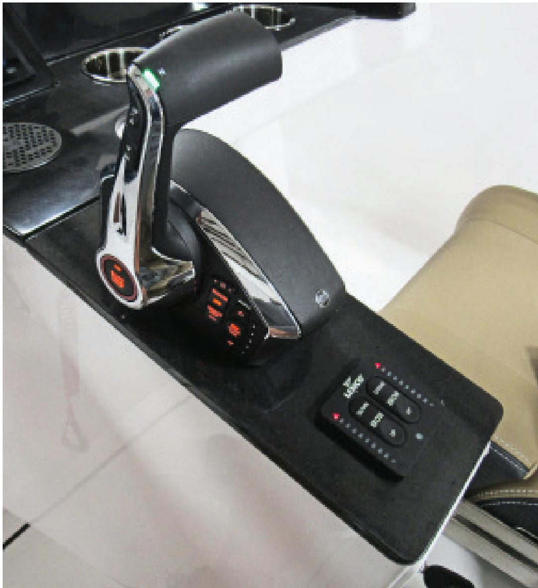
Single Engine Control And Trim Tab Switches With Indicators
