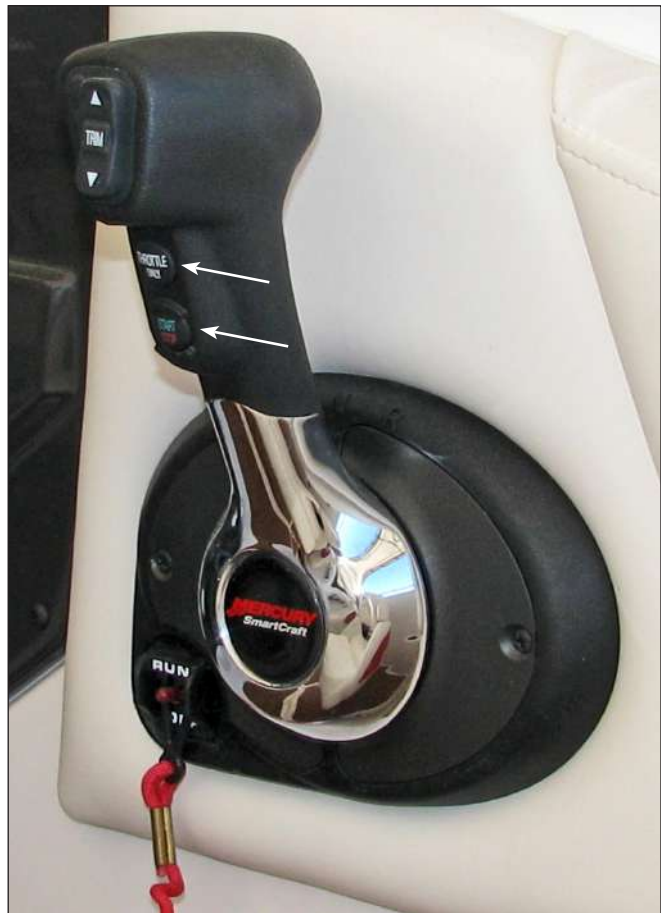
Typical Mercury Electronic Control & Switches
