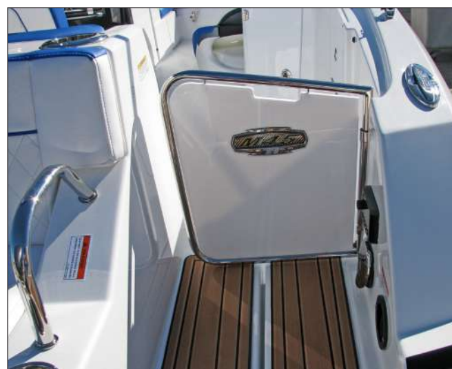
Transom Door Closed (Door must be in the open position before the aft cockpit hatch can be raised)
