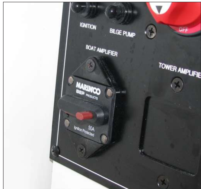
Battery Switch Panel & Optional Amplifier Circuit Breaker
