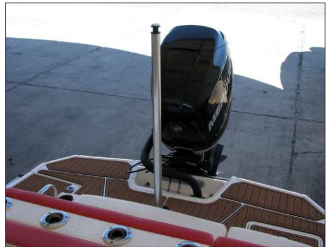
Ski Tow Pylon
