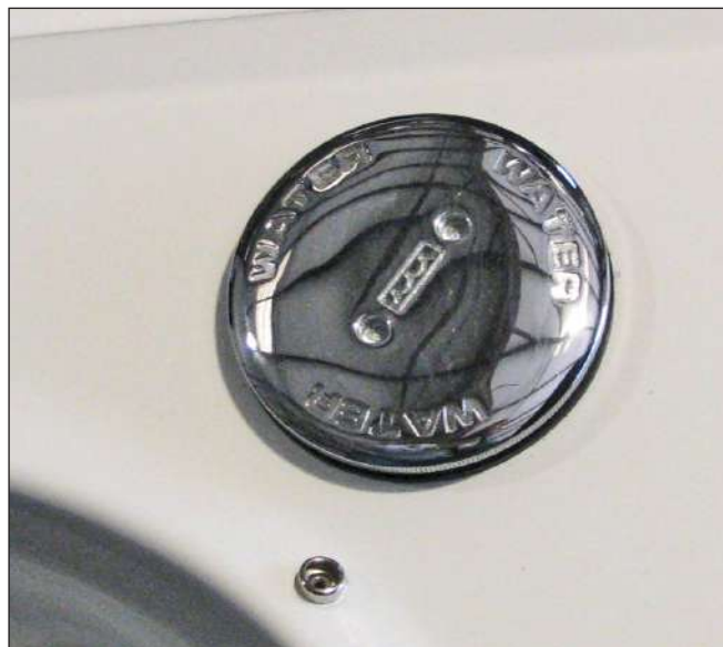
Fresh Water Fill
