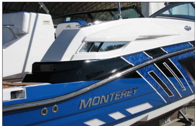
Bilge Compartment Vents
