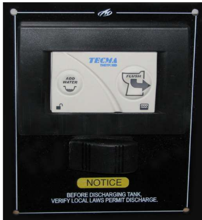
Electric Head Control Panel In Head Compartment
