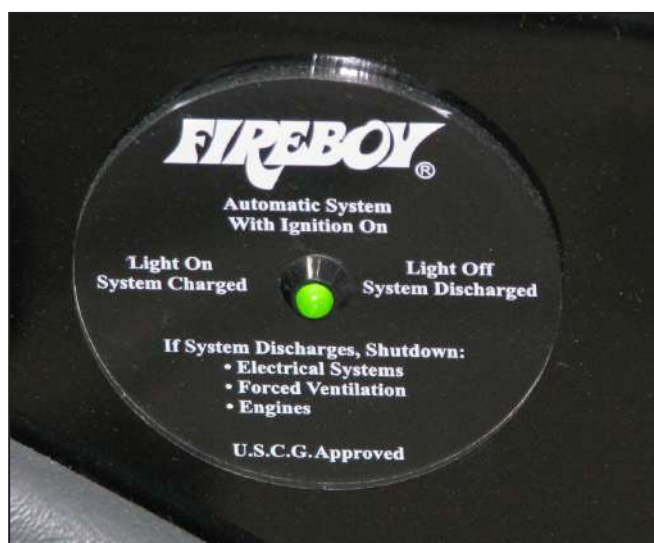
Fire Extinguisher Panel In Helm
