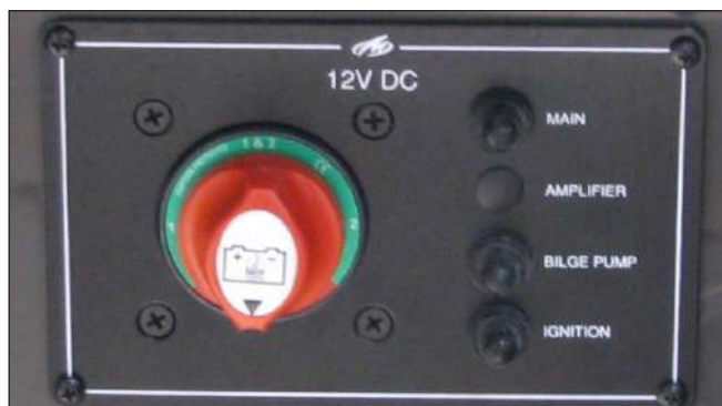
Typical 268SS Dual Battery Switch Panel
