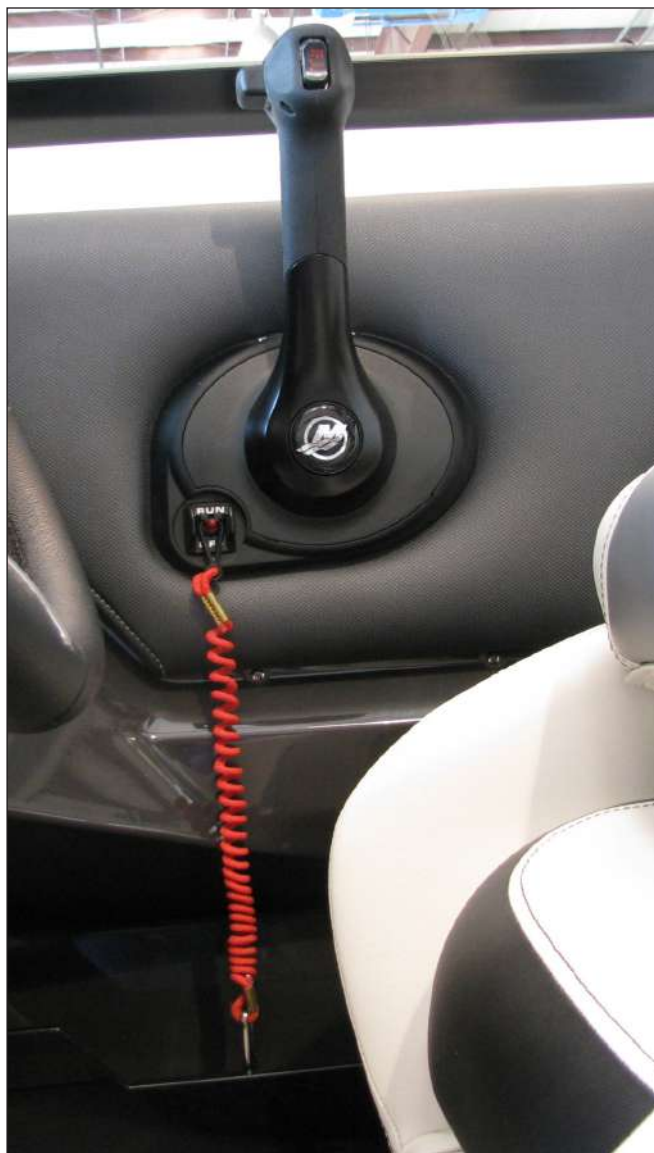
Mercruiser Control Emergency Stop Switch & Lanyard
