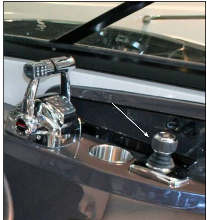
Typical Mercruiser DTS Joystick Control
