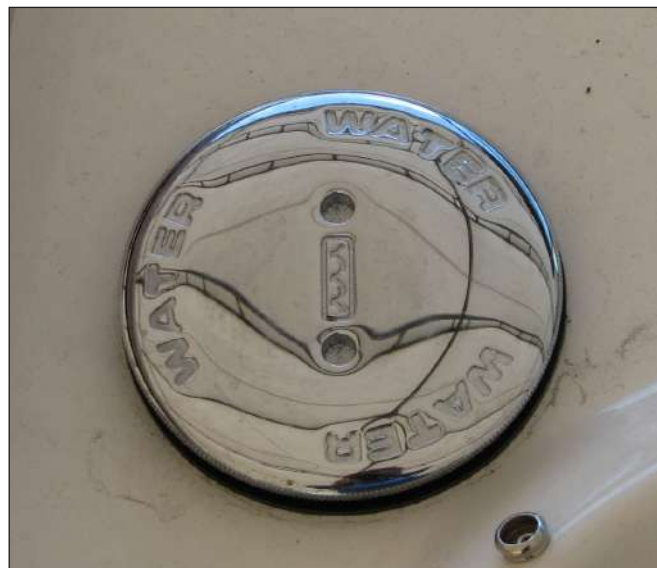
Fresh Water Fill
