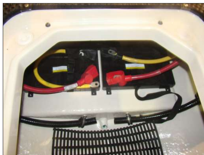
In-Floor Storage Compartment Battery Mounting Location 214SS/218SS & 234SS/238SS
