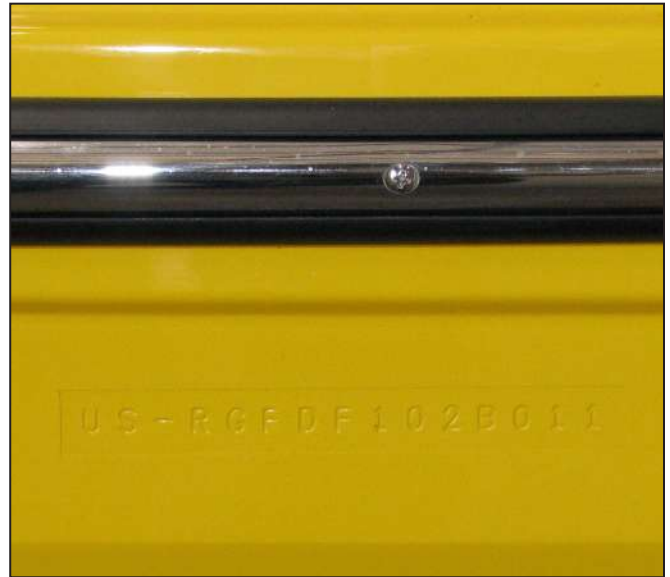
Hull ID # On Starboard Side of Transom
