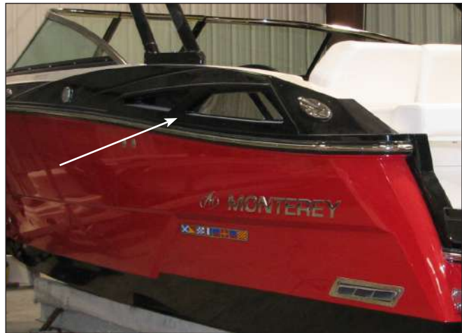
Typical Engine Compartment Vents
