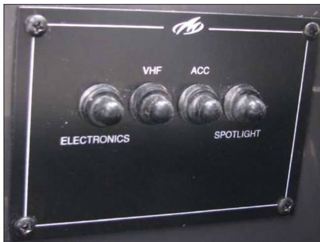
288SS & 328SS Helm Accessory Breaker Panel
