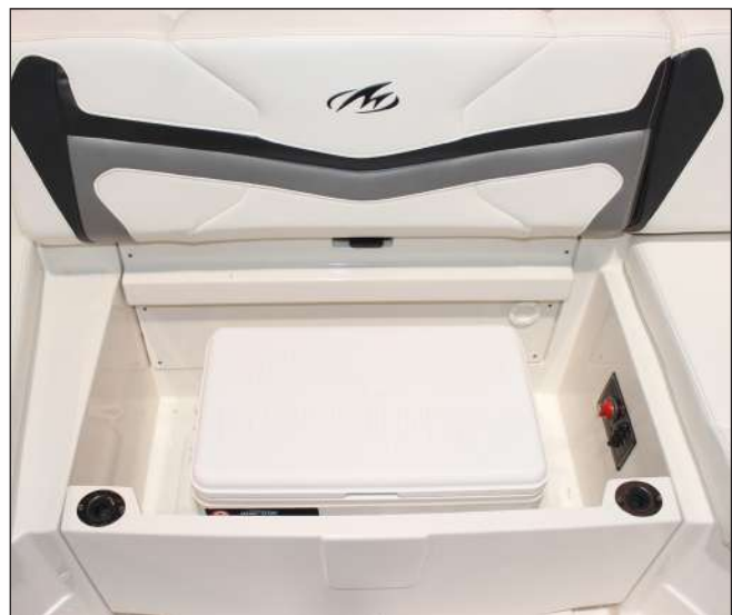
Cooler/Battery Switch/Fire Port Compartment 214SS/218SS & 234SS/238SS
