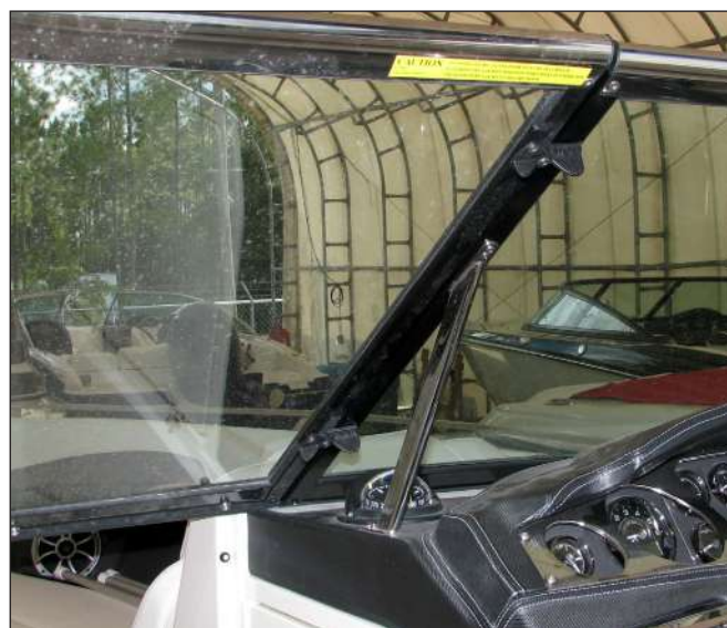
288SS Windshield Center Section Latches
