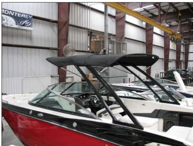
Arch With Front & Rear Top Sections
