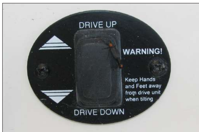
Typical Outdrive Tilt Switch Near Transom Door
