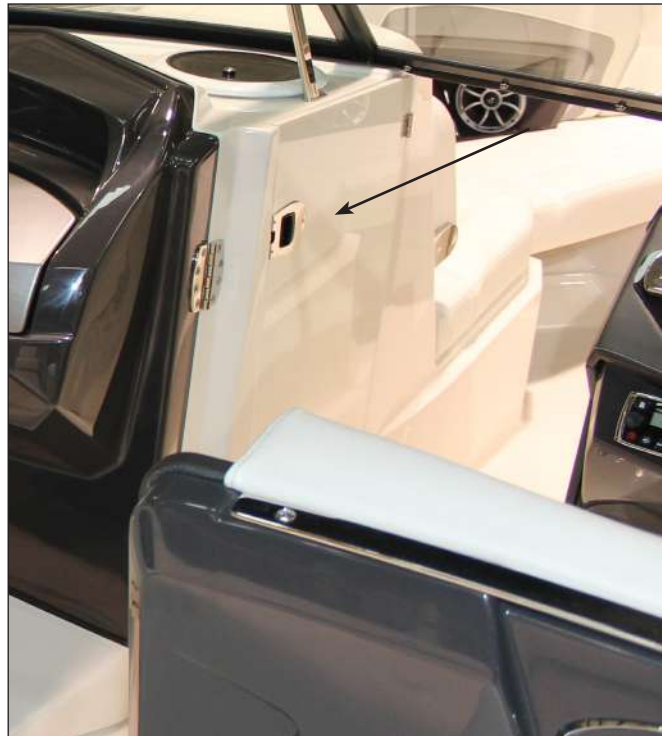
288SS Walk-through Door Latched In The Open Position
