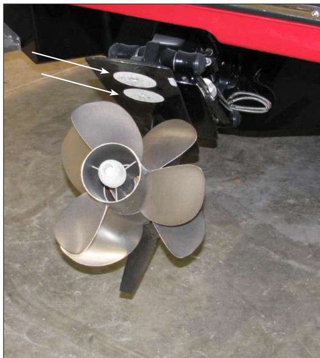
Typical Mercruiser Outdrive Anodes
