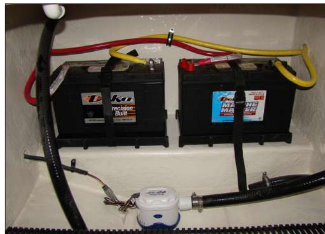
288SS Forward Automatic Bilge Pump
