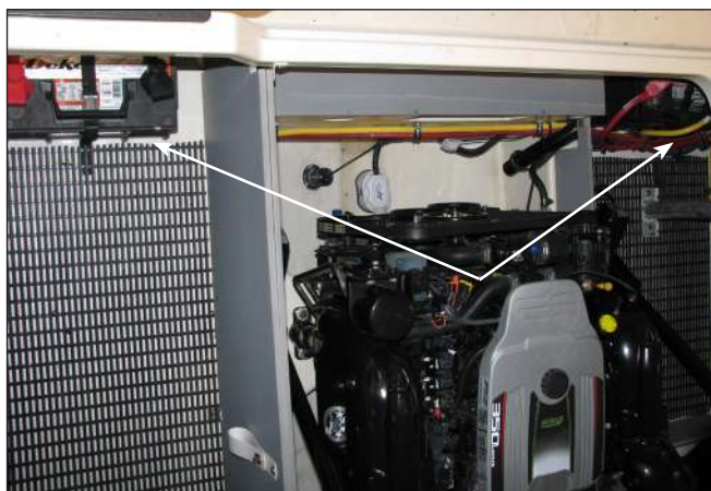
268SS Dual Battery Mounting Location In Engine Compartment
