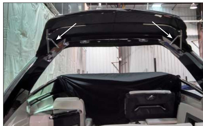
Rear Top Stretched Tight With Adjustable Stanchions on Each Side of Main Bow
