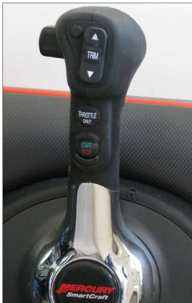
Mercuriser Single Engine Tilt/Trim Switch
