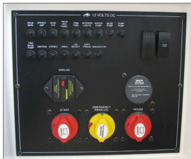
288SS Dual Battery Switch Panel & Circuit Protection
