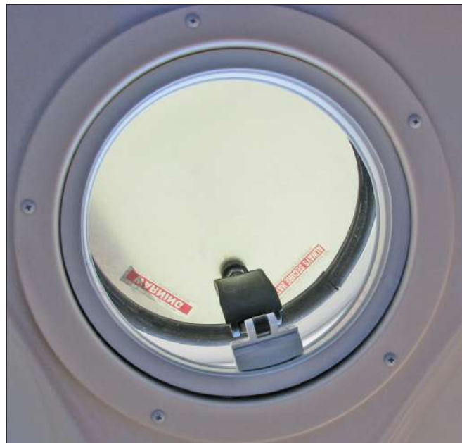
288SS Head Compartment Hatch Closed
