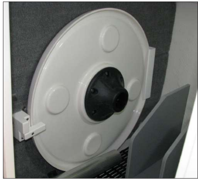
268SS Table Secured With Rotating Latch
