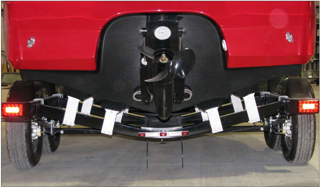
Trailer Bunks - Supporting Hull Properly
