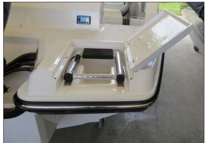
Boarding Ladder In Compartment
