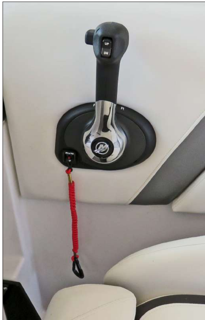
Mercury Engine Control, Emergency Stop Switch & Lanyard
