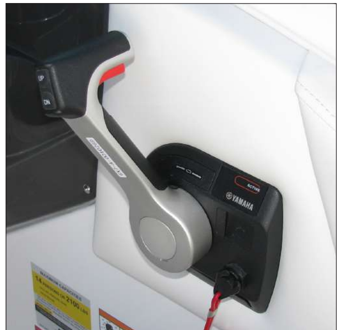
Typical Yamaha Engine Side Mount Electronic Control & Emergency Stop Switch
